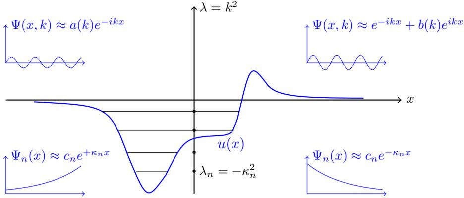
Figure 1: The time-independent scattering problem. The small graphs show the asymptotic behaviour of the eigenfunctions  $\Psi_n(x)$  and  $\Psi(x, k)$  in the corresponding regions. For  $\lambda < 0$ , only exponentially decaying solutions are feasible in order to be normalizable. For  $\lambda > 0$ , we consider an incoming wave from the right whose amplitude is set to 1.
