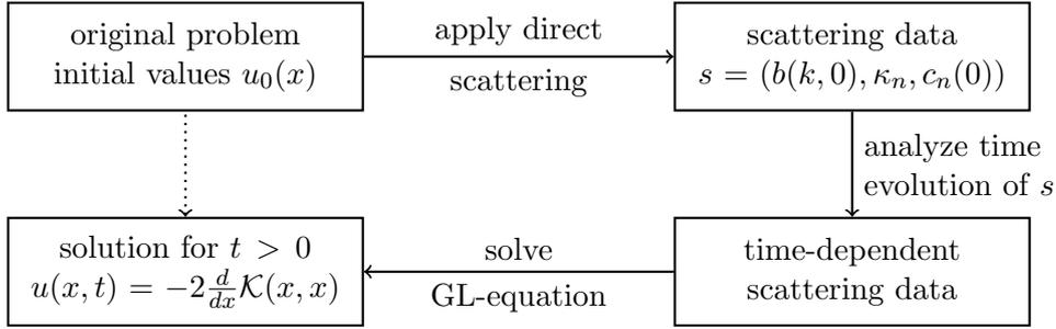
Figure 2: Schematic illustration of the inverse scattering transform
